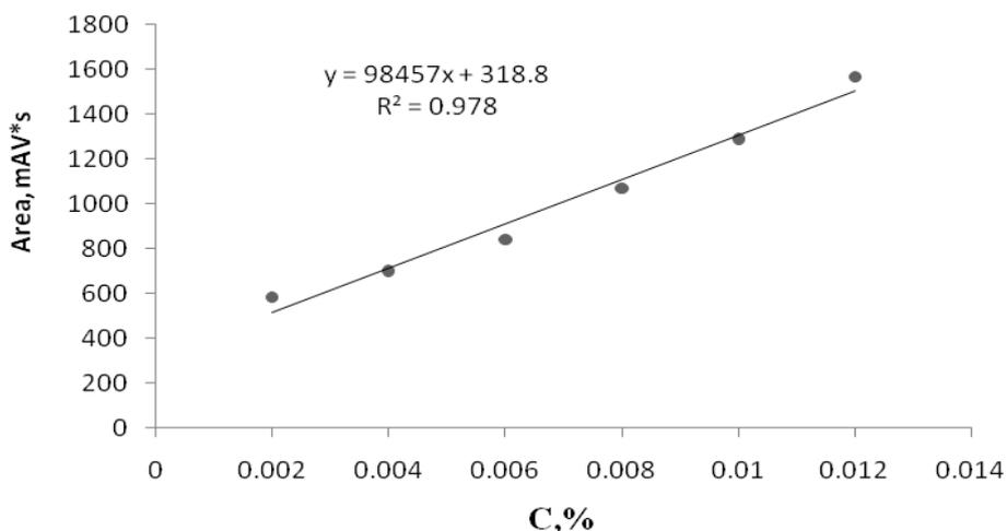
Figure 3: The calibration plot of the peak area of the concentration of standard sample routine.
