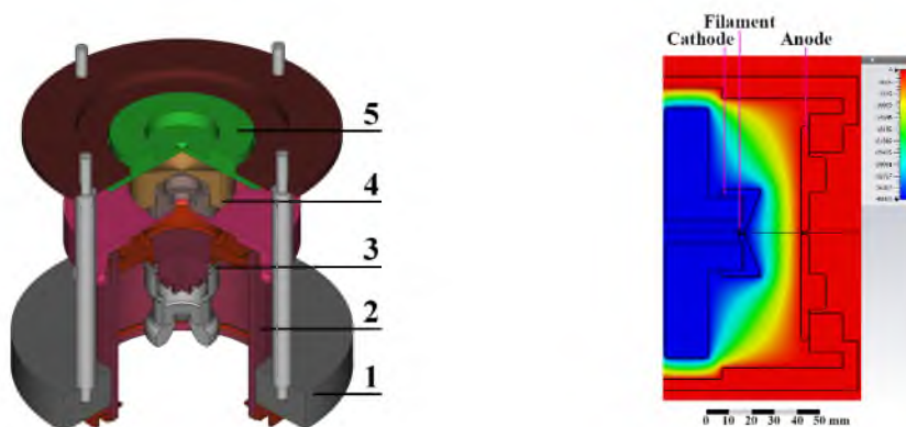
Figure 2. 3D image of the electron gun (left) and example of potential distribution (right): 1 — mounting flange, 2 — insulator, 3 — HV connector, 4 — cathode (HV electrode), 5 — anode.
