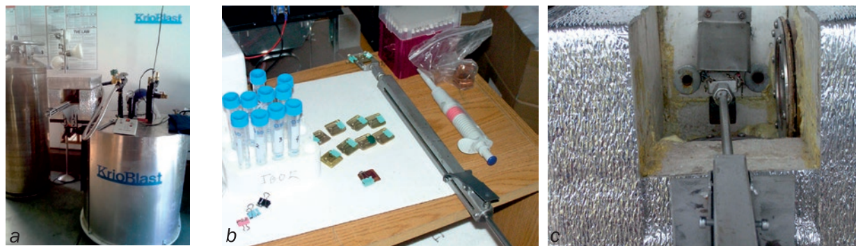
Fig. 2. General view of KrioBlast TM -2 system (a), cryogenic containers VitriPlates TM -2 filled with different concentrations of glycerol (b), and Speargun plunger in the “released” position (c).
