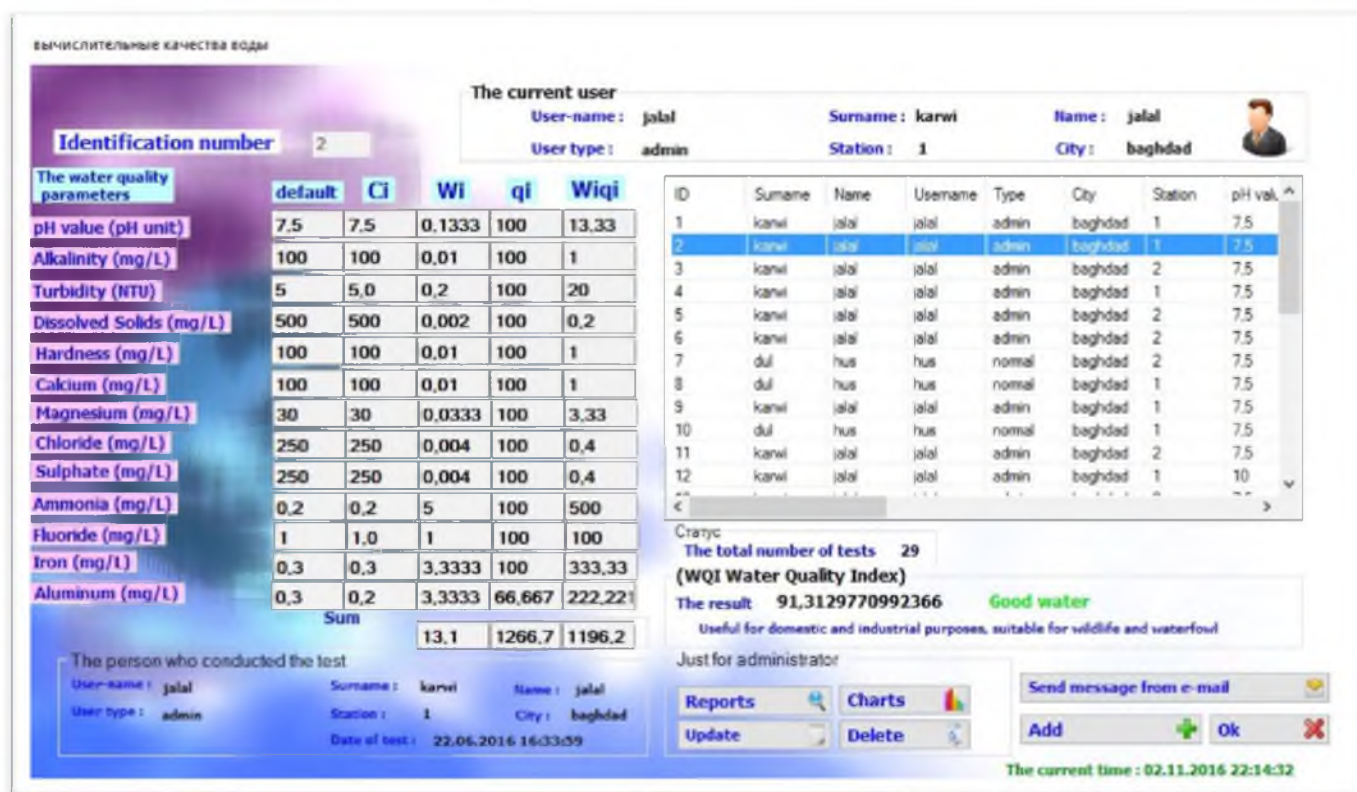
Fig. 3. Main window of data analysis and modeling for water quality calculation
