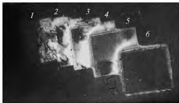
Fig. 1. Fragment of the liquid-crystal cell with the silicon substrate irradiated by a focused ion beam under scanning conditions. The irradiation dose is (1) 3.1 \times 10^{14} , (2) 9.3 \times 10^{14} , (3) 1.86 \times 10^{15} , (4) 3.72 \times 10^{15} , (5) 7.44 \times 10^{15} , and (6) 1.48 \times 10^{16} ions/cm 2 .
