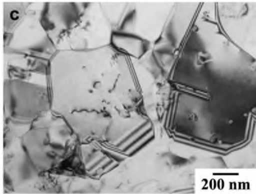
Fig. 8. Microstructure of a Ni-20%Cr alloy strained to \varepsilon \sim 6.5 and annealed at 600 °C for 1 h. (a) Typical OIM picture; white and black lines correspond to subgrain/grain boundaries with misorientations of 2^\circ \leq \theta < 15^\circ and 15^\circ \leq \theta , respectively; (b) misorientation distribution of (sub)grain boundaries; (c) TEM image of recrystallized grains.
