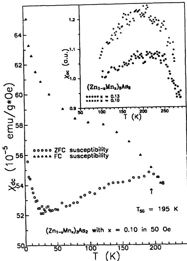
Fig. 2. Spin-glass like behaviour of ZMA  $x = 0.10$ . The maximum in the ZFC curve at  $T_f = 195$  K can easily be seen. The inset shows the ac-susceptibilities of the  $x = 0.10$  and  $0.13$  samples, measured at the frequency of 320 Hz and the driving field of 0.7 Oe.
