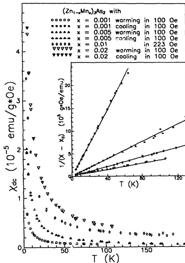
Fig. 1. DC-susceptibility of ZMA for  $x \leq 0.05$ . Open and closed symbols indicate the ZFC- and FC-samples, respectively. The inset shows a Curie-Weiss fit of the results.
