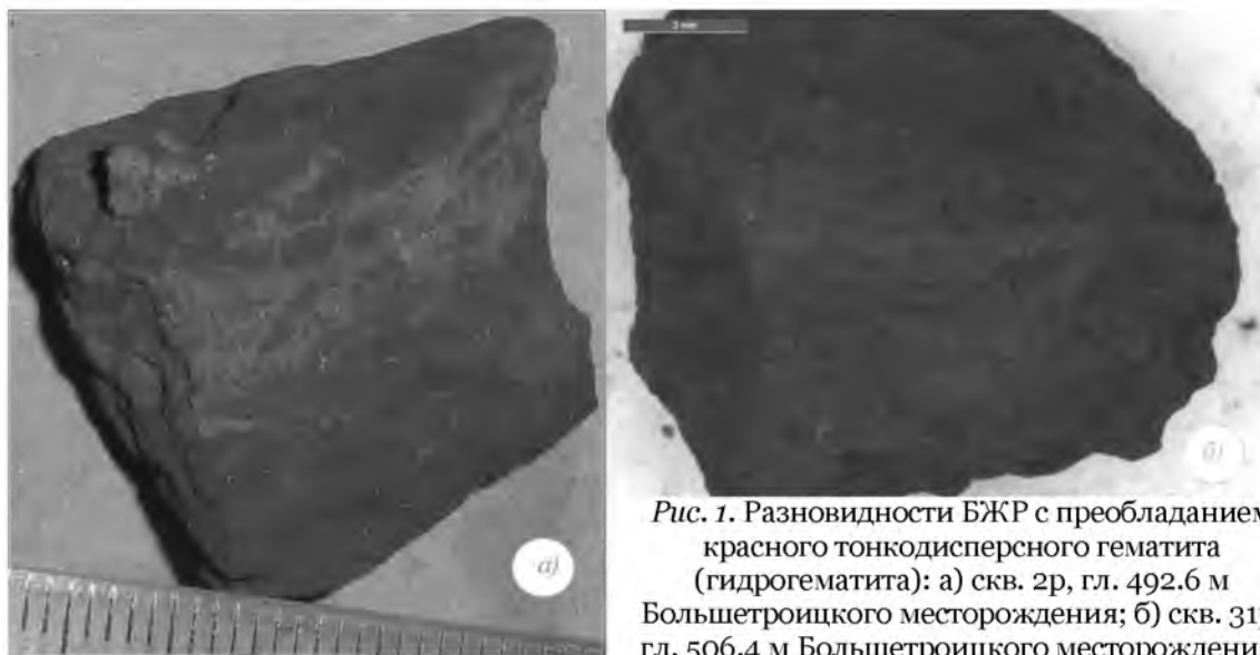
Fig. 1. Types of high-grained hematite ores: a) well 2R, depth 492.6 m; b) well 31R, depth 506.4 m; white interlayers – berthierine
