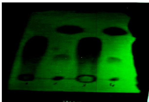
Figure 1. TLC chromatogram for partially purified cinnamic acid under UV radiation at 254 nm.
