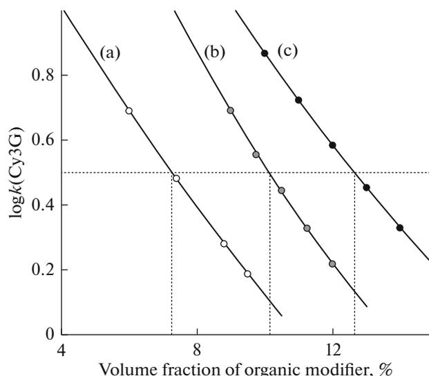
**Fig. 1.** Effect of organic modifier concentration on the retention of cyanidin-3-glucoside in three eluent systems: (a) 10 vol % formic acid–(6–10) vol % acetonitrile–water; (b) 1 vol % orthophosphoric acid–(10–20) vol % acetonitrile–water; and (c) 1 vol % orthophosphoric acid–(10–15) vol % ethanol–water.
