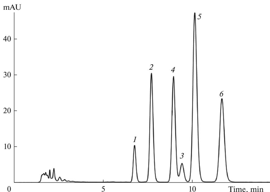
**Fig. 5.** Separation of six different cyanidin 3-glucosides in a mobile phase of composition 11.2 vol % ethanol–1 vol % orthophosphoric acid–87.8 vol % water. Mobile phase flow rate 0.8 mL/min, temperature 40°C, column 150 × 4.6 mm Symmetry C18, 3.5 μm. Anthocyanins: (1) Cy3Sopho, (2) Cy3GRut, (3) Cy3G, (4) Cy3Sam, (5) Cy3XRut, and (6) Cy3Rut.
