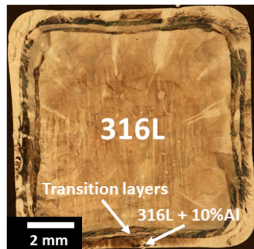
Fig. 5 The appearance of the as-printed gradient material
